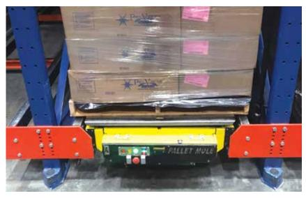
The Pallet Mole® was utilized for over 150,000 cubic feet of space comprised of 76 bays of rack with 22 pallet deep aisles at the Nor-Am facility. (Photo courtesy of Frazier Industrial Company.)
