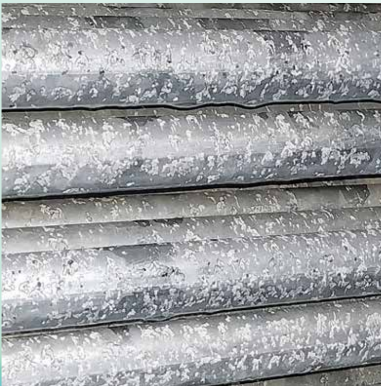
White Rusted Coil without Pass-Protect
