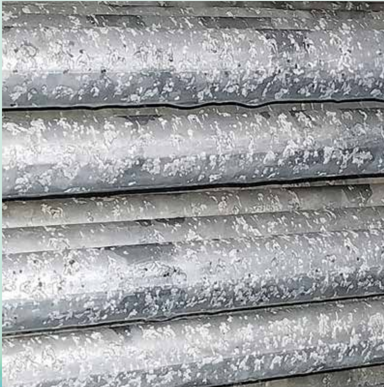
White Rusted Coil without Pass-Protect
