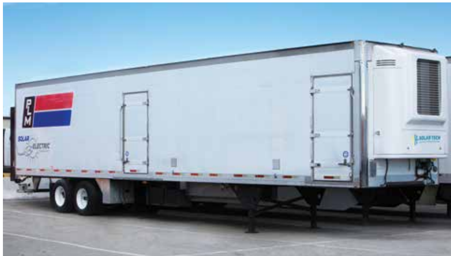
PLM Fleet offers a hybrid-electric TRU and a zero-emission eTRU solution. (Photo courtesy of PLM Fleets.)
