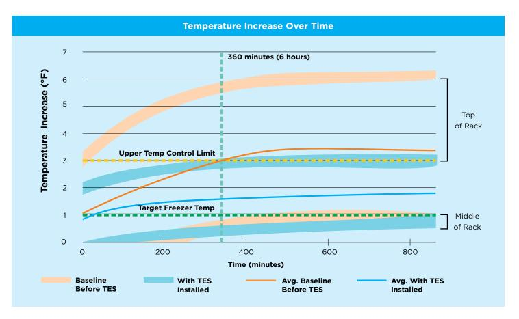
Thousands of individual temperature data points are illustrated in the chart above. The shaded bands represent the range of temperatures recorded, and the solid lines represent the average temperature in the room.
