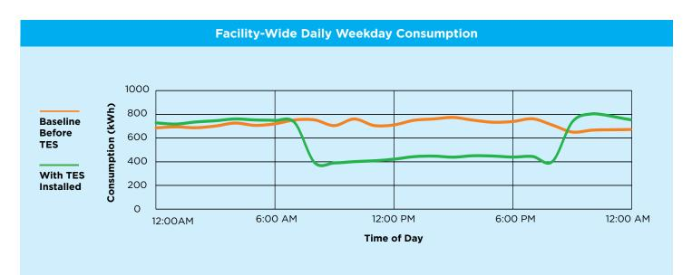
When measuring the decrease in energy usage of just the freezers where the TES was installed and in operation, refrigeration energy consumption was reduced by 35%. The expensive peak period hours were targeted for reduction to maximize dollar savings. Peak period kWh consumption across the entire study period was reduced by 43%.
