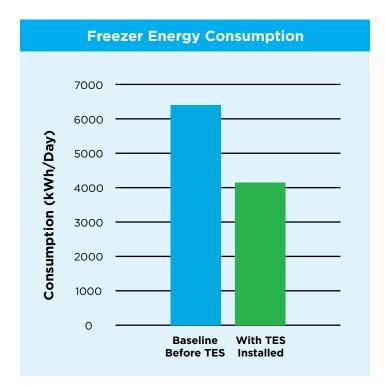
Looking at total energy consumption across the entire facility, post implementation of the TES system the entire facility experienced a weekday energy consumption reduction of 20%. This was slightly offset by a 5% increase in off-peak weekend consumption by the freezer in order to fully recharge the TES modules in preparation for the following week. The net result was a 13% reduction of energy consumption for the entire facility each week.
